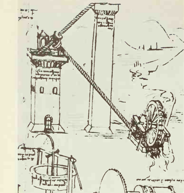
62. LEFT Archimedean screws for bringing water to the top of a tower in two stages
